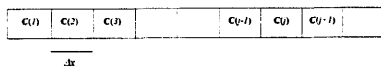
Fig. 2. Discrete model of the solution in an electrochemical experiment considering only linear diffusion.
